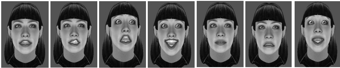
Fig. 6. Examples of a single-frame LUCIA’s emotive expressions. These were obtained by acquiring real movements with ELITE, by automatically tracking and reconstructing them with “TRACK” and by reproducing them with LUCIA.
