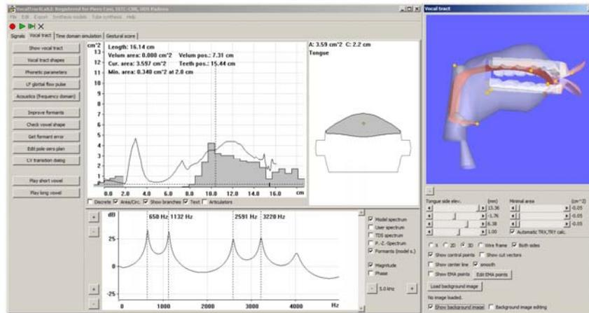
The shape and/or position of the articulators is defined by a number of vocal tract parameters, which can be changed interactively by dragging some control points (see the dots in the vocal tract picture in Figure 3). The pictures on the right side of Figure 3 display the cross section through the vocal tract at a selected position along the centerline (top), and the vocal tract area function (bottom). At the bottom of the screen is a graph of the volume velocity transfer function.
